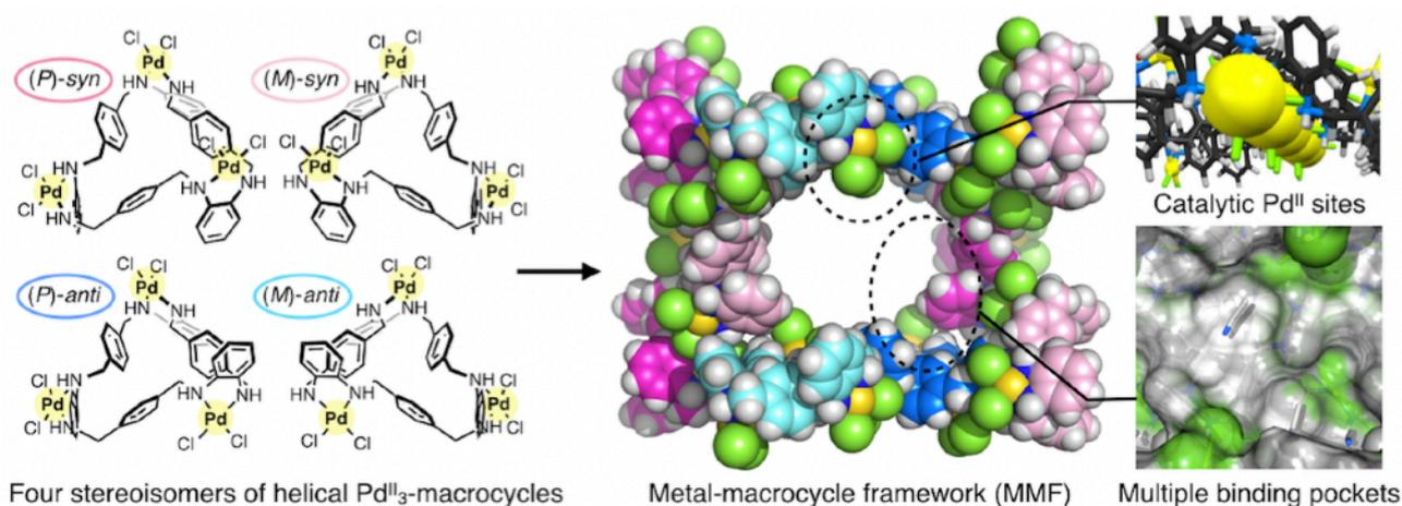
**Figure 1** Formation and structure of metal-macrocycle framework (MMF)
