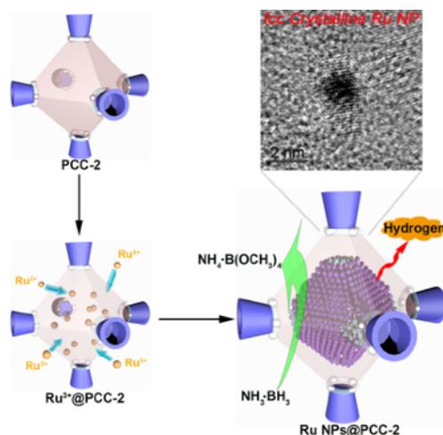
**Figure 1** *fcc* Ru nanoparticle encapsulated within porous coordination cage.
